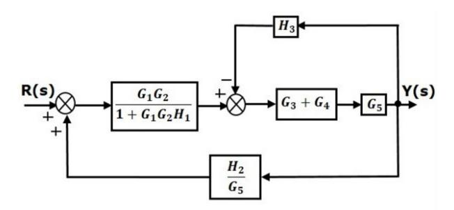
**Step 3** – Use Rule 1 for blocks  $(G_3 + G_4)$  and  $G_5$ . The modified block diagram is shown in the following figure.
