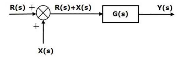
Summing point has two inputs  $\ R(s)$  and  $\ X(s)$  . The output of it is  $\ \{R(s)+X(s)\}$  .
