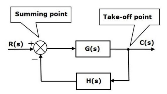
The above block diagram consists of two blocks having transfer functions G(s) and H(s). It is also having one summing point and one take-off point. Arrows indicate the direction of the flow of signals. Let us now discuss these elements one by one.
