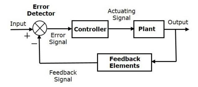
The error detector produces an error signal, which is the difference between the input and the feedback signal. This feedback signal is obtained from the block (feedback elements) by considering the output of the overall system as an input to this block. Instead of the direct input, the error signal is applied as an input to a controller.
