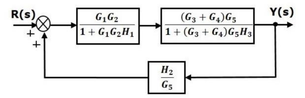
**Step 5** – Use Rule 1 for blocks connected in series. The modified block diagram is shown in the following figure.
