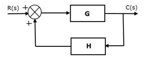
The concept of transfer function will be discussed in later chapters. For the time being, consider the transfer function of positive feedback control system is,
