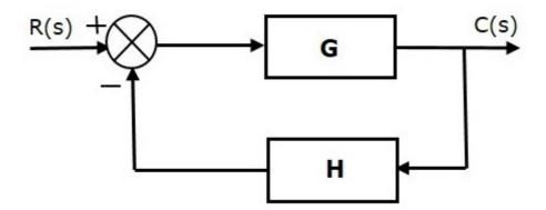
Transfer function of negative feedback control system is,
