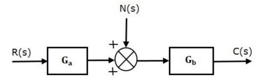
The open loop transfer function due to noise signal alone is
