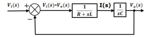
Similarly, you can draw the **block diagram** of any electrical circuit or system just by following this simple procedure.
