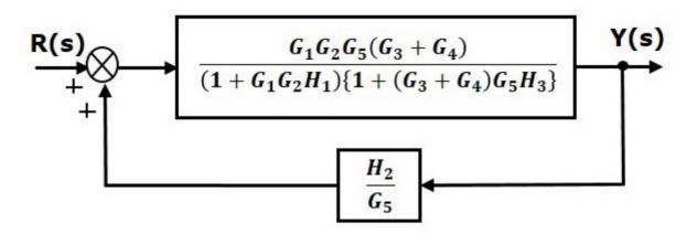
**Step 6** – Use Rule 3 for blocks connected in feedback loop. The modified block diagram is shown in the following figure. This is the simplified block diagram.
